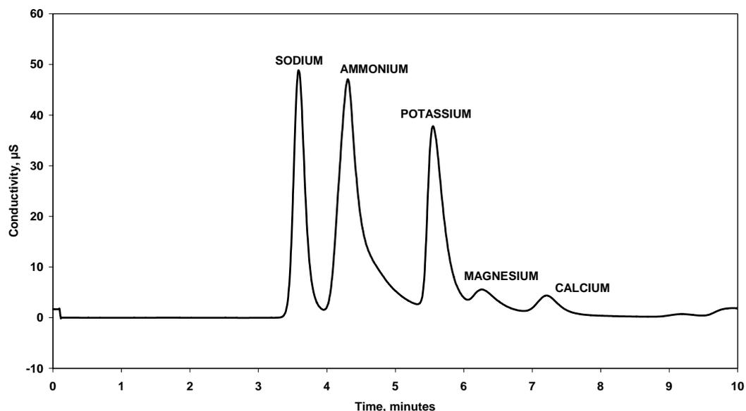
**Figure 1:** Example chromatogram showing the peaks related to each cation.
